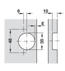
For screw fixing Drilling pattern 48/6
